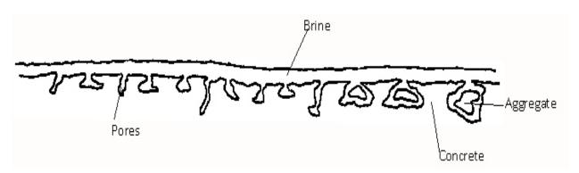
With "SALT" based products, including Sodium Chloride, Potassium Chloride and Magnesium Chloride, the Brine formed has a freezing point in the region of -10°C to -15°C, with SPIT FIRE the freezing point is below -36°C.
